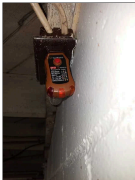
Some outlets throughout the house tested as open ground
