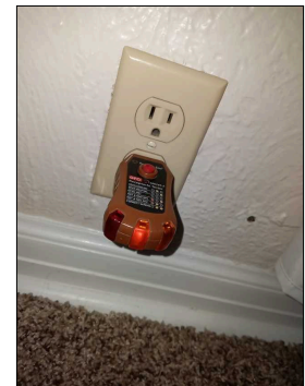
Some outlets throughout the house tested as open ground
